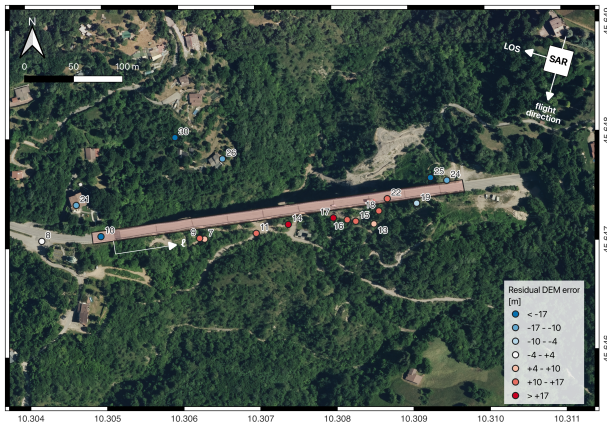
Figure 2. Spatial distribution of PS surrounding the Lumezzane viaduct, color-coded by the estimated topographic error ( \Delta h ). A systematic lateral shift is evident between the PS corresponding to the structure (red-ish points) and the actual optical footprint of the deck. This spatial offset is a predictable geometric consequence of projecting elevated scatterers onto a bare-earth reference DEM during the interferometric geocoding process.
