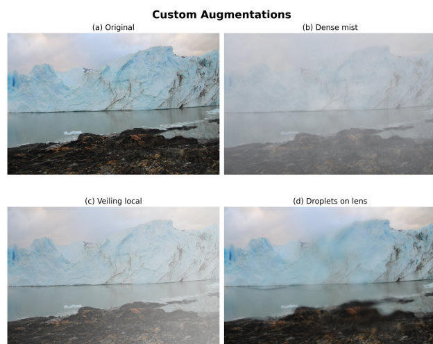
Figure 2. Custom environment oriented augmentations: (a) original image, (b) dense mist with reduced visibility and contrast, (c) local veiling simulating mist onset, and (d) droplet-based distortion simulating lens contamination.
