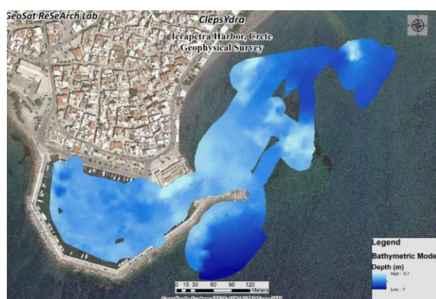
Figure 5. Digital bathymetric model of Lerapetra harbor resulted by the sonar survey.
