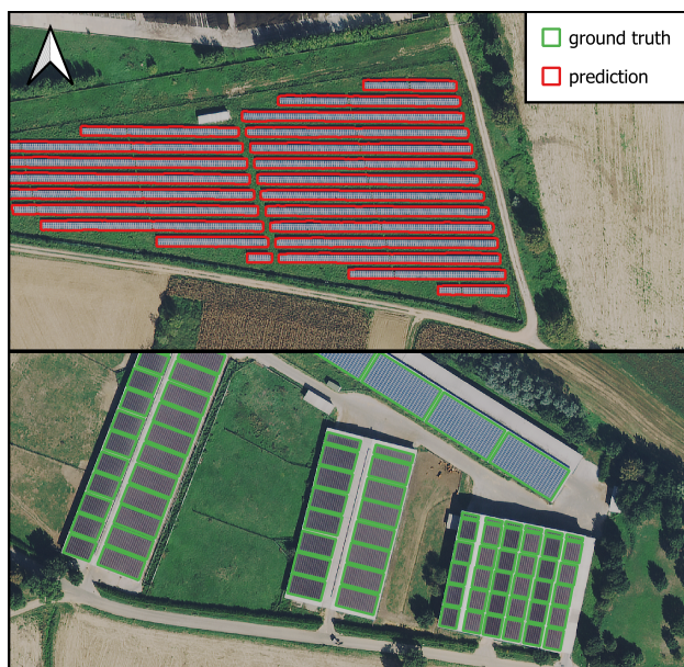
Figure 7. Missing ground truth annotations but found with YOLO11-m (top), Roof mounted PV panels and corresponding ground truth (bottom).
