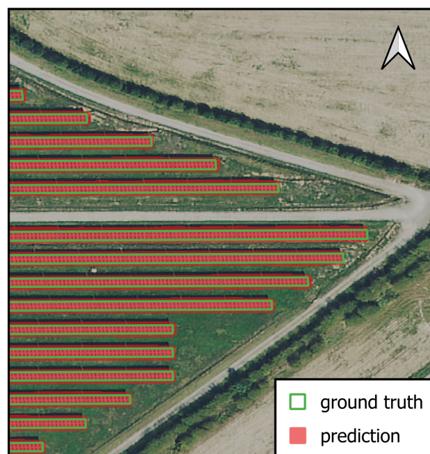
Figure 6. Example YOLO prediction and ground truth for the Piedmont dataset.
