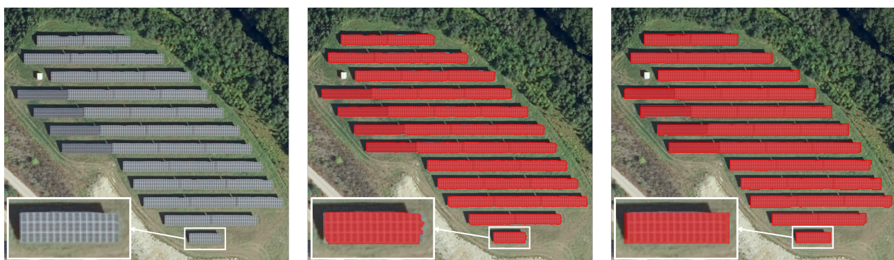
Figure 5. Segmentation result of a ground-mounted photovoltaic system (left: DOP20, centre: U-Net result, right: YOLO result).
