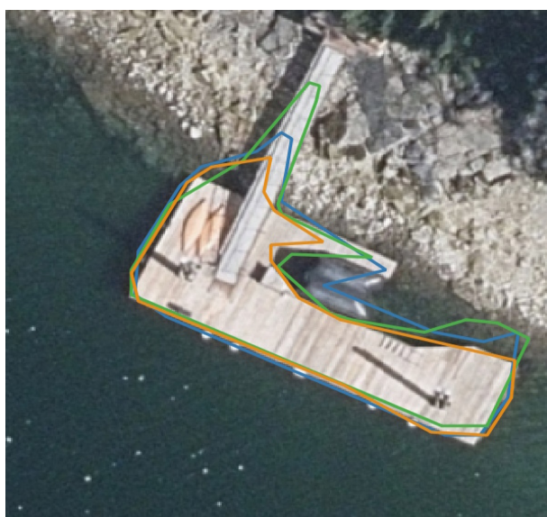
Figure 3. Example dock outlines for raw (green), scan-angle (blue), and range-corrected (orange) intensity domains.
