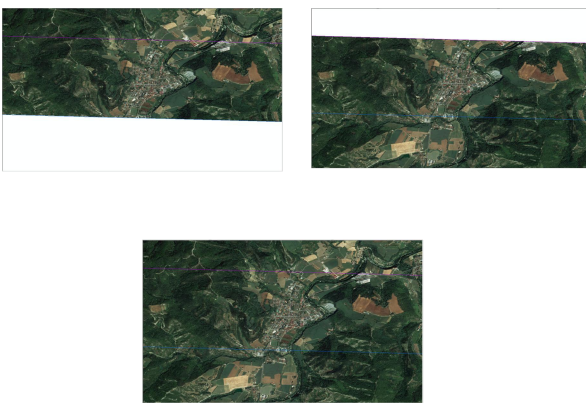
Figure 6 The above two are adjacent tiles to be fused, with obvious null values. The following is the effect after tile fusion
