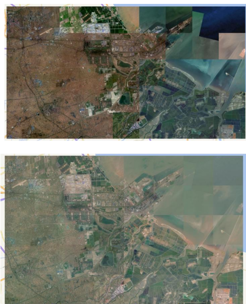
Figure 5 Comparison chart before and after color balance. The above image is before calibration, and the following image is after calibration.
