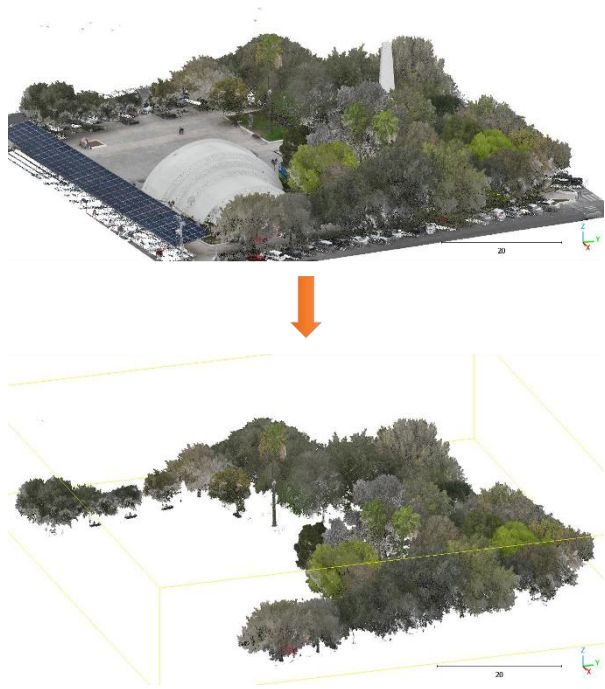
Figure 5. (a) Raw 3D LiDAR point cloud of UGA-1 and (b) non-ground points extracted using the Cloth Simulation Filter (CSF) algorithm. The filtering process separates terrain points from vegetation returns
