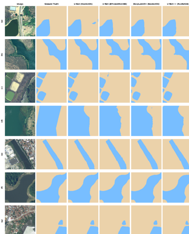
Figure 3. Water segmentation results using aerial imagery
