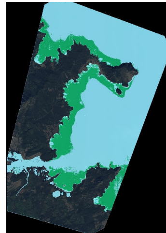
Figure 8. Classified 2021 Neo-Pléiades multispectral image, through the SVM algorithm. Land is shown in black, sea in light blue, and Posidonia oceanica in green.
