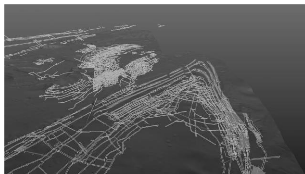
Figure 9. Example 3D visualisation of underground workings digitised from historical documentation.
