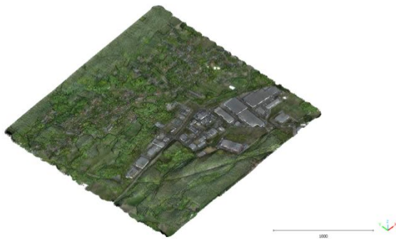
Figure 4. The final point cloud prepared for analysis, thinned using an Octree-based method.
