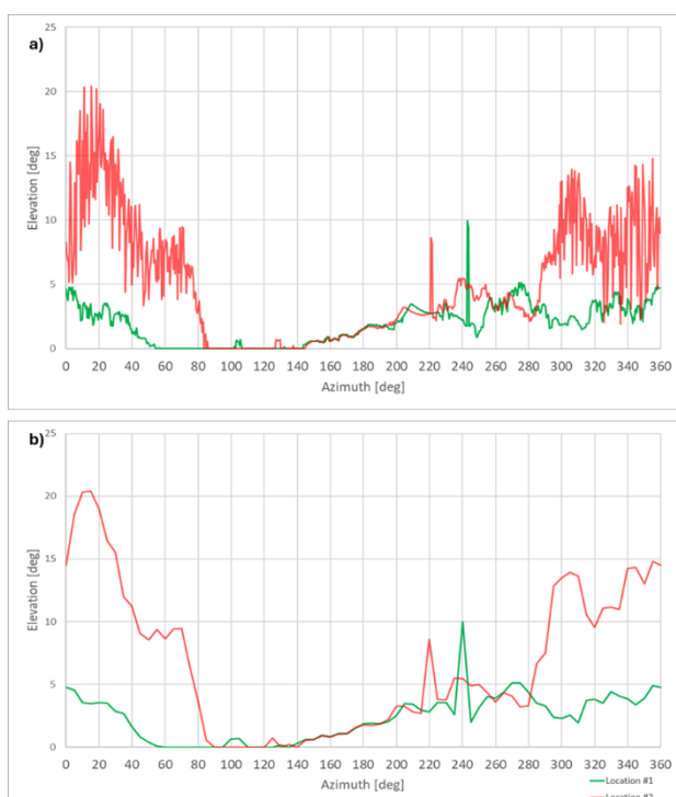
Figure 7. Examples of elevation mask visualization as a line plot for both analyzed locations and a planned antenna height of 15 m AGL. Similarly to the radar plot, the 0.5° angular interval (a) provides a much more faithful representation of actual obstacles compared to the generalized 5° interval (b).
