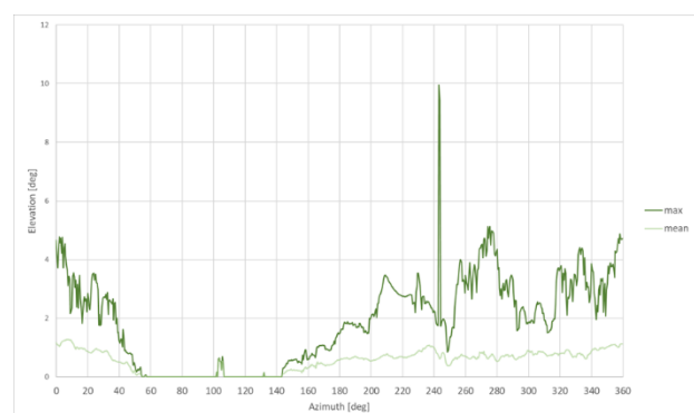
Figure 9. The difference between the elevation mask generated using the MAX and MEAN functions for location #1 and an antenna height of 15 m AGL.
