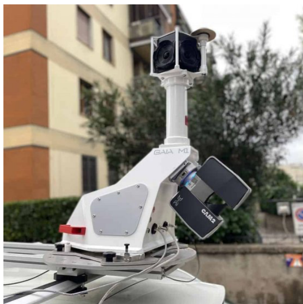
Figure 2. The GAIA M1 mobile mapping system installed on the survey vehicle.
