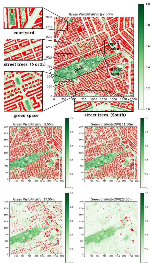
Figure 9. Results of Green visibility Index (GVI). The red areas represent the building voxels at each height layer, the green areas represent the GVI values at each voxel location.
