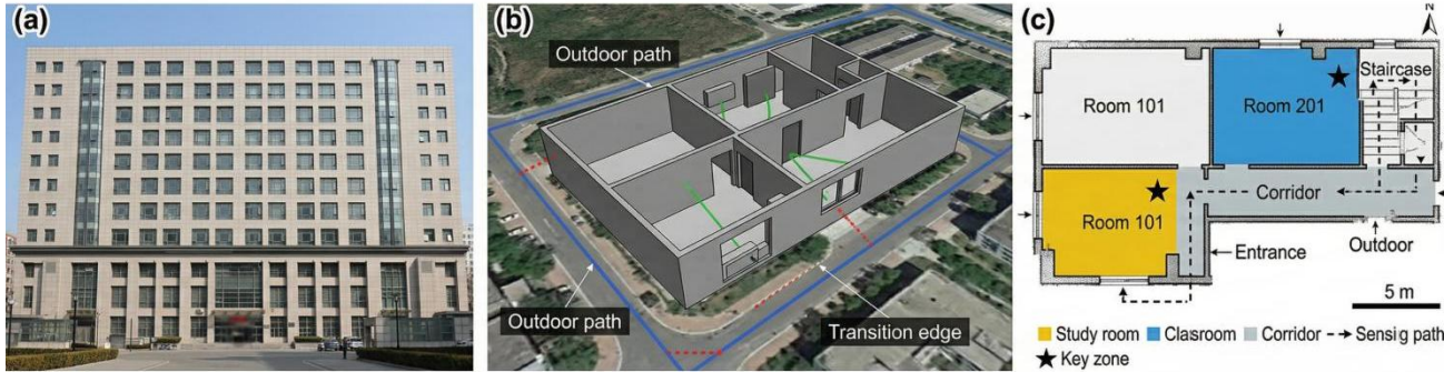
Fig. 4. Experimental site and digital twin model. (a) Exterior photograph of the teaching building; (b) Cesium platform screenshot showing the integrated LOD4 indoor model with outdoor road network and topological edges (blue: outdoor paths, green: indoor connections, red dashed: transition edges at entrances); (c) Annotated floor plan derived from the SLAM point cloud horizontal cross-section, with color-coded functional zones (yellow: 1F study room, blue: 2F classrooms, gray: corridors) and the sensing kit traversal path (arrows).
