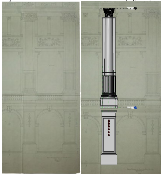
Figure 7. Parametric family modeling of the columns on the west elevation of the France pavilion, based on a layout drawing, original scale 1:10 (Archivio Stefano Molli - Fondazione Marazza).
