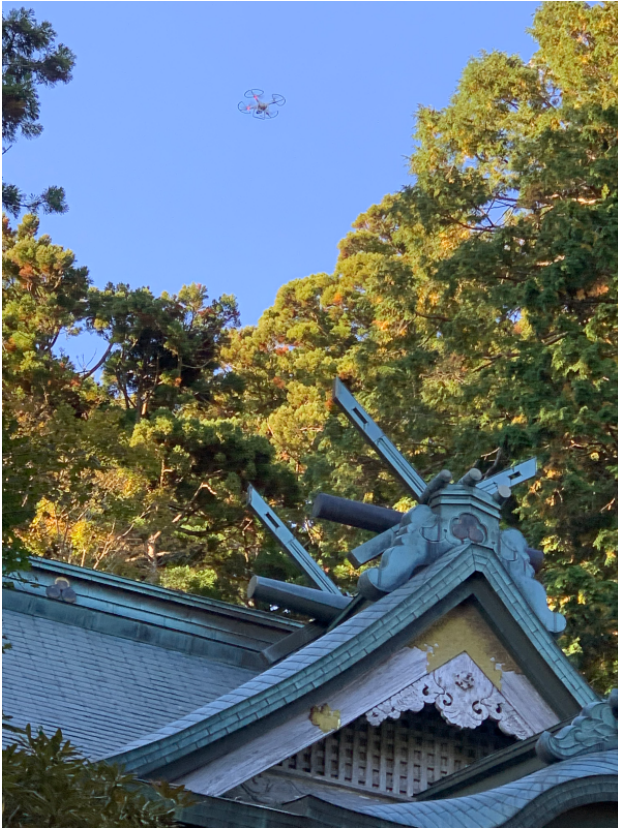
Figure 3. Photogrammetry using a drone to capture high-altitude geometric details of the roof
