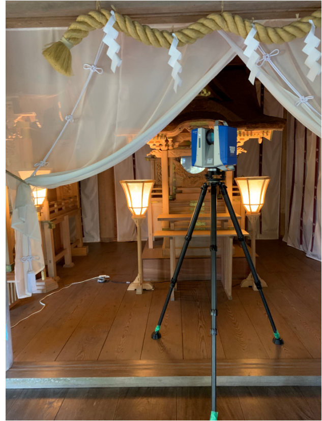
Figure 2. Terrestrial laser scanning of the shrine's main hall
