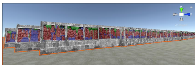
Figure 5. Torch-based Level of Detail (LoD) optimisation in Unity. Objects within the illumination radius are rendered in full resolution; distant regions are progressively simplified, reducing render batch count by over 35%.
