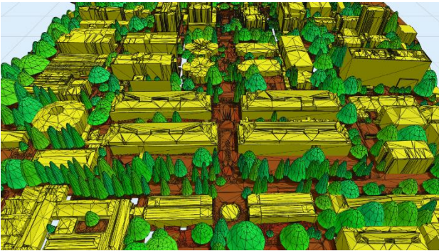
Figure 4. Instance-level semantic mesh derived from CityGML through citygml2obj conversion.
