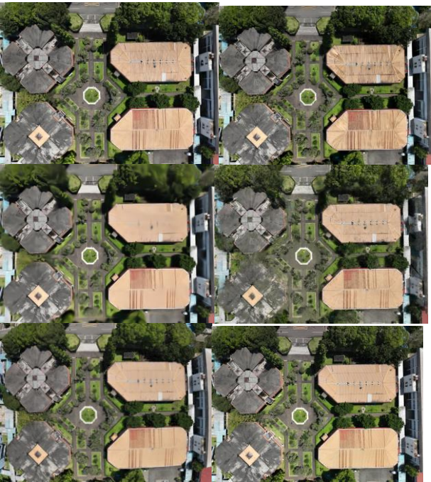
Figure 6. Rendered views from identical input camera poses: (a, top-left) Postshot (Splat3), (b, top-right) Lichtfeld Studio (MRNF), (c, middle-left) CLM-GS, (d, middle-right) Triangle Splatting, (e, bottom-left) Photorealistic Mesh, and (f, bottom-right) References.
