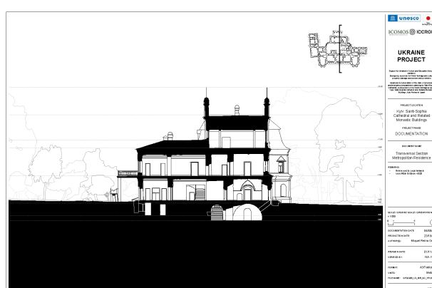
Figure 11. Traced section from point cloud data.
