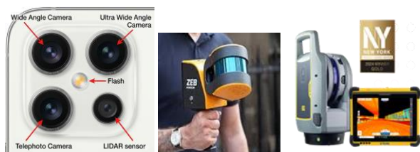
Figure 3. Instruments used in this study. Left: iPhone 12 Pro with integrated dToF LiDAR, wide, ultra-wide, and telephoto cameras; Middle: GeoSLAM ZEB Horizon handheld SLAM scanner; Right: Trimble X9 terrestrial laser scanner.
