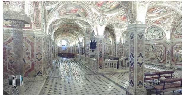
Figure 4. Point cloud acquired by Faro Focus 3D s120 and processed in the proprietary software Faro Scene
