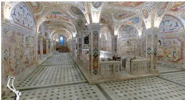
Figure 6. Point cloud acquired by NavVis VLX and processed in NavVis IVION
