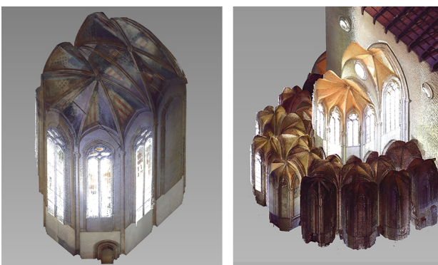
Figure 10. Data acquisition – S. Lorenzo and Donnaregina point cloud from laser scanner
