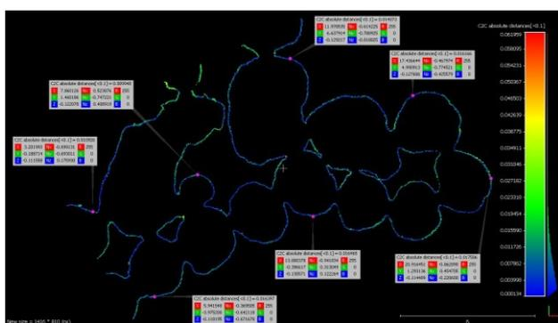
Figure 8. Rooms 10 -18 to 27: C2C analyses of horizontal slices between the P30 and BLK2GO point clouds (calculation range: 0.00-0.02 m).
