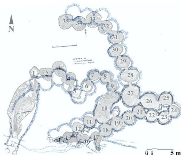
Figure 6. Overlap between the orthophoto, in grey, obtained by P30-BLK2GO final point cloud (2021) and, in blu, two-dimensional representation of Guzzardi (1980).
