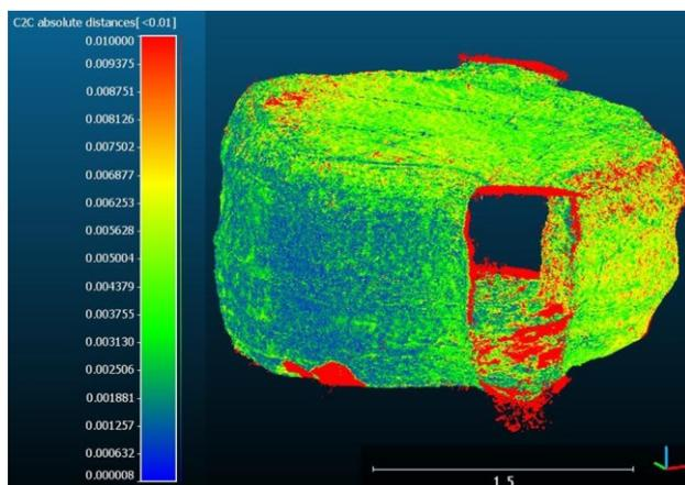
Figure 11. Room 23: C2C analyses between the P30 and GoPro point clouds (calculation range: 0.00-0.01 m).
