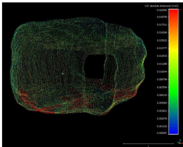
Figure 10. Room 23: C2C analyses between the P30 and BLK2GO point clouds (calculation range: 0.00-0.02 m).
