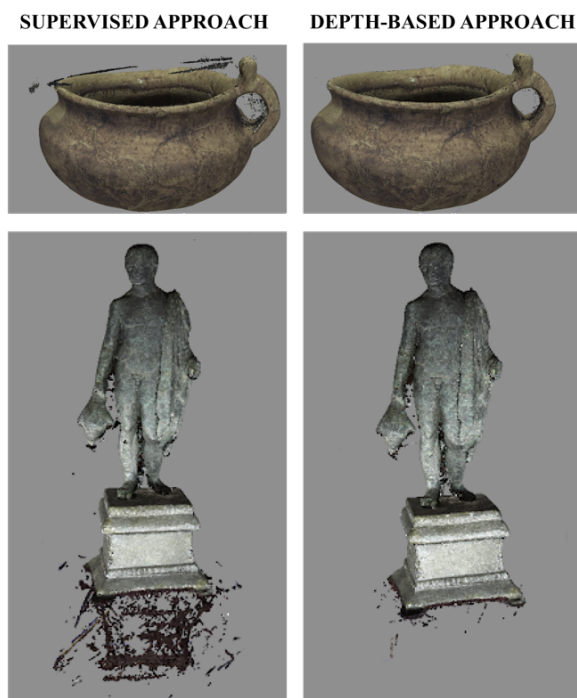
Figure 9. Dense point cloud results applying image masks within the MVS reconstruction process.
