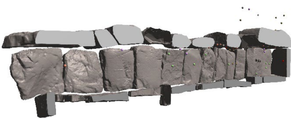
Figure 7. Display of the points of interest: microbiological samples in green, sensors in purple and the remaining of former interventions in orange
