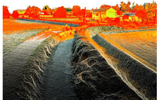
Figure 3. Point cloud integrated between MLS and drone photogrammetry. Second case study: irrigation systems of the agricultural system of the Pavia plain.
