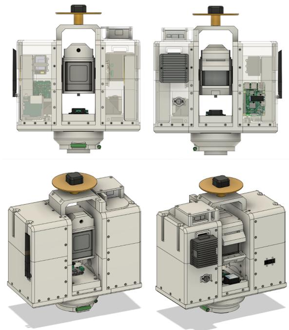
Figure 3. 3D CAD model of the developed TLS
