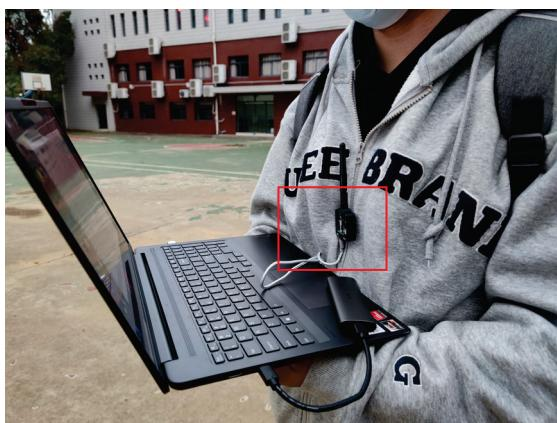
**Figure 6.** UWB tag installation.
