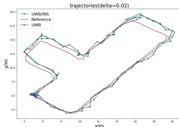
**Figure 8.** Comparison of reference trajectory, UWB trajectory, and UWB/INS integration trajectory when  $\delta_0 = \delta_1 = \delta_2 = 0.02$  ( $\delta_0, \delta_1, \delta_2$  are the diagonal elements of the observation noise covariance matrix).
