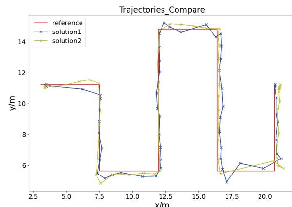
**Figure 7.** Comparison of the reference trajectory and the trajectory obtained by the two base station arrangements of ‘solution 1’ and ‘solution 2’.
