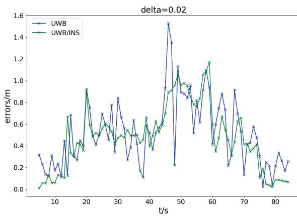
**Figure 9.** Comparison of the positioning error of UWB and the positioning error of UWB/INS integration when  $\delta_0 = \delta_1 = \delta_2 = 0.02$  ( $\delta_0$ ,  $\delta_1$ ,  $\delta_2$  are the diagonal elements of the observation noise covariance matrix).
