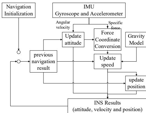
**Figure 1.** INS mechanization process.
