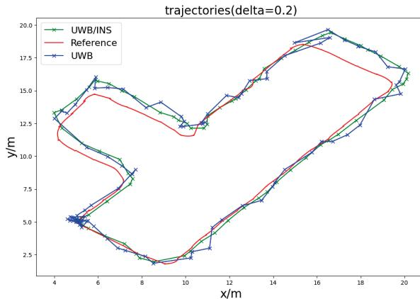
**Figure 10.** Comparison of reference trajectory, UWB trajectory, and UWB/INS integration trajectory when  $\delta_0 = \delta_1 = \delta_2 = 0.2$  ( $\delta_0$ ,  $\delta_1$ ,  $\delta_2$  are the diagonal elements of the observation noise covariance matrix).
