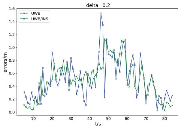
**Figure 11.** Comparison of the positioning error of UWB and the positioning error of UWB/INS integration when  $\delta_0 = \delta_1 = \delta_2 = 0.2$  ( $\delta_0$ ,  $\delta_1$ ,  $\delta_2$  are the diagonal elements of the observation noise covariance matrix).
