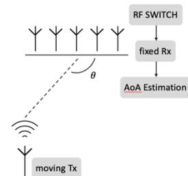
Figure 1. Bluetooth 5.1 AoA mechanism.
