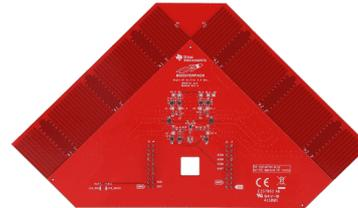
**Figure 3.** SimpleLink™ Angle of Arrival BoosterPack.
