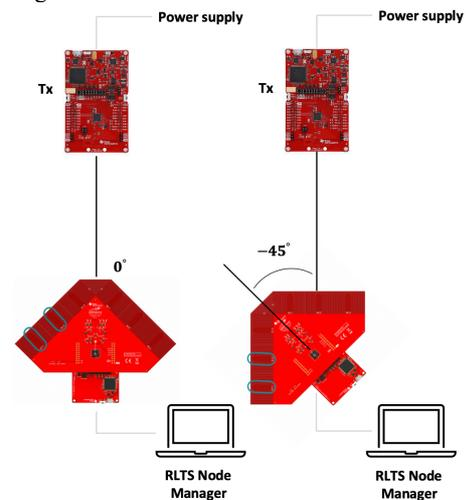
**Figure 12.** Placement of BLE devices at the angle of 0°, -45°.
