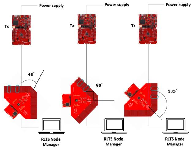
**Figure 6.** Device placement at the angle of 45°, 90°, 135°.
