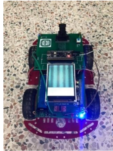
Figure 7. Receiving terminal platform
