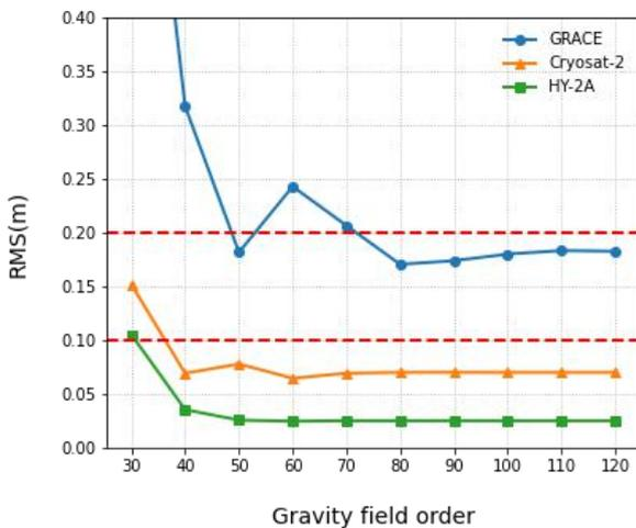
**Figure 5.** RMS(m) in radial direction for different orders in 30 minutes prediction.
