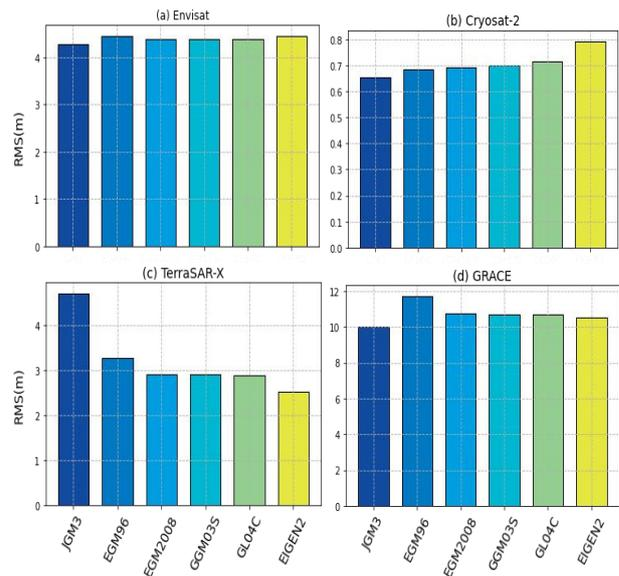
**Figure 3.** Comparison of 3-days different satellite orbits prediction precision with the different gravity models.
