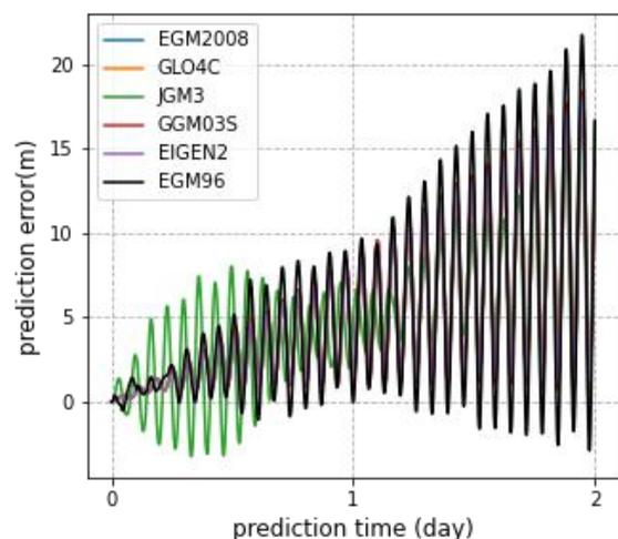
**Figure 4.** The GRACE satellite orbit prediction error (radial direction) in 1st Jan 2012.
