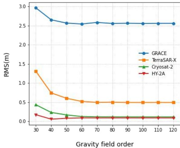
**Figure 6.** LEO Orbit Prediction Error in the radial direction of different satellites for different orders for 1-day prediction.
