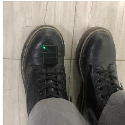
**Figure 5.** IMU tied on the left foot.
