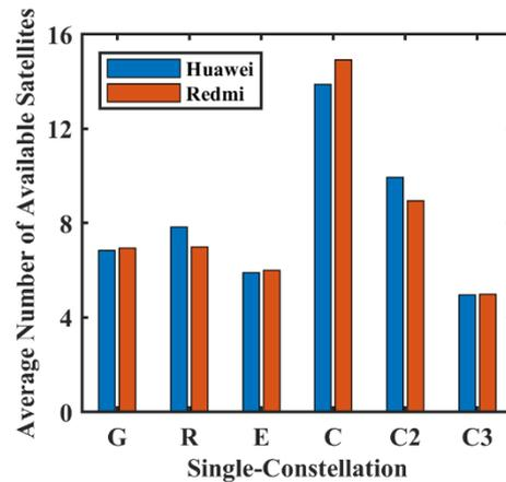
Figure 13. The average number of available satellites for single-constellation in velocity determination
