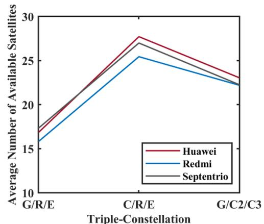
Figure 3. The average number of available satellites for velocity determination in triple-constellation.
