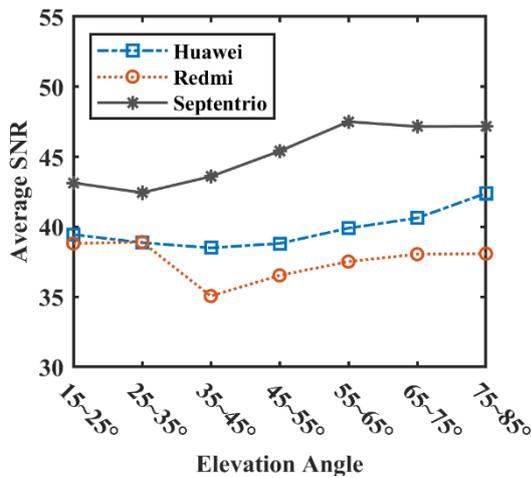
Figure 4. Average SNR for different angles of altitude.
