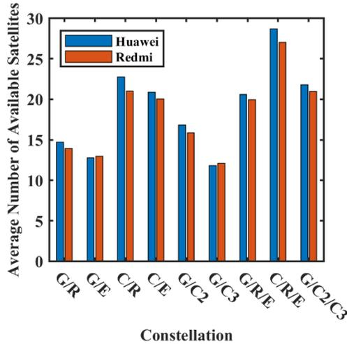
Figure 15. The average number of available satellites for dual/triple-constellation in velocity determination.
