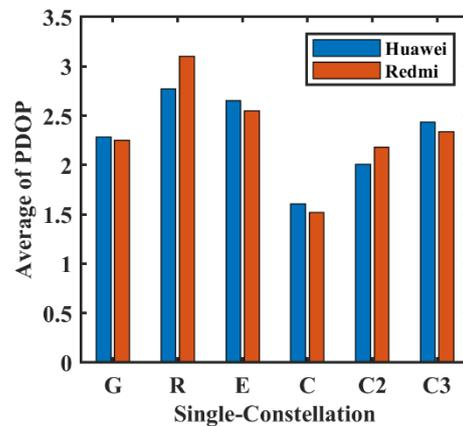
Figure 14. The average PDOP for single-constellation in velocity determination.
