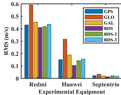
Figure 6. RMS histogram of velocity determination errors in vertical directions of single-constellation.
