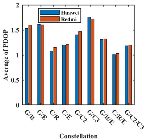
Figure 16. The average PDOP for dual/triple-constellation in velocity determination.
