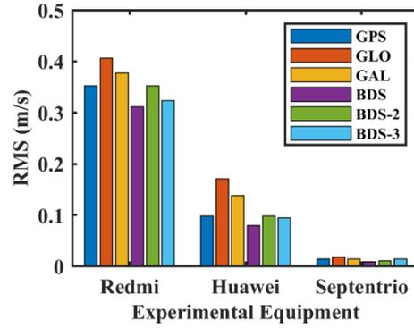
Figure 5. RMS histogram of velocity determination errors in horizontal directions of single-constellation.
