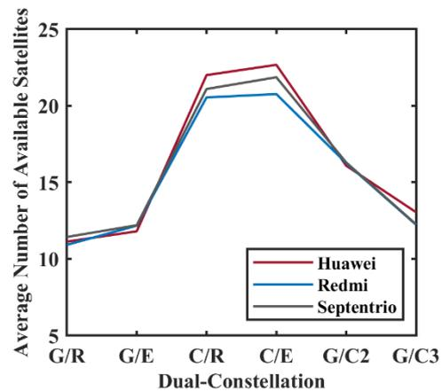
Figure 2. The average number of available satellites for velocity determination in dual-constellation.
