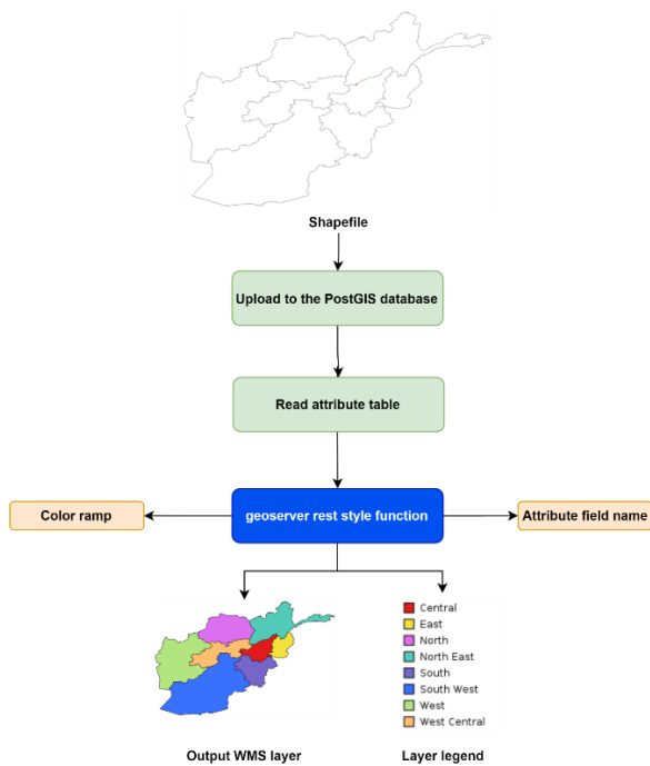
Figure 7. Process of generation of WMS layer of raster dataset using geoserver-rest. The input data is the administrative regions of Afghanistan
