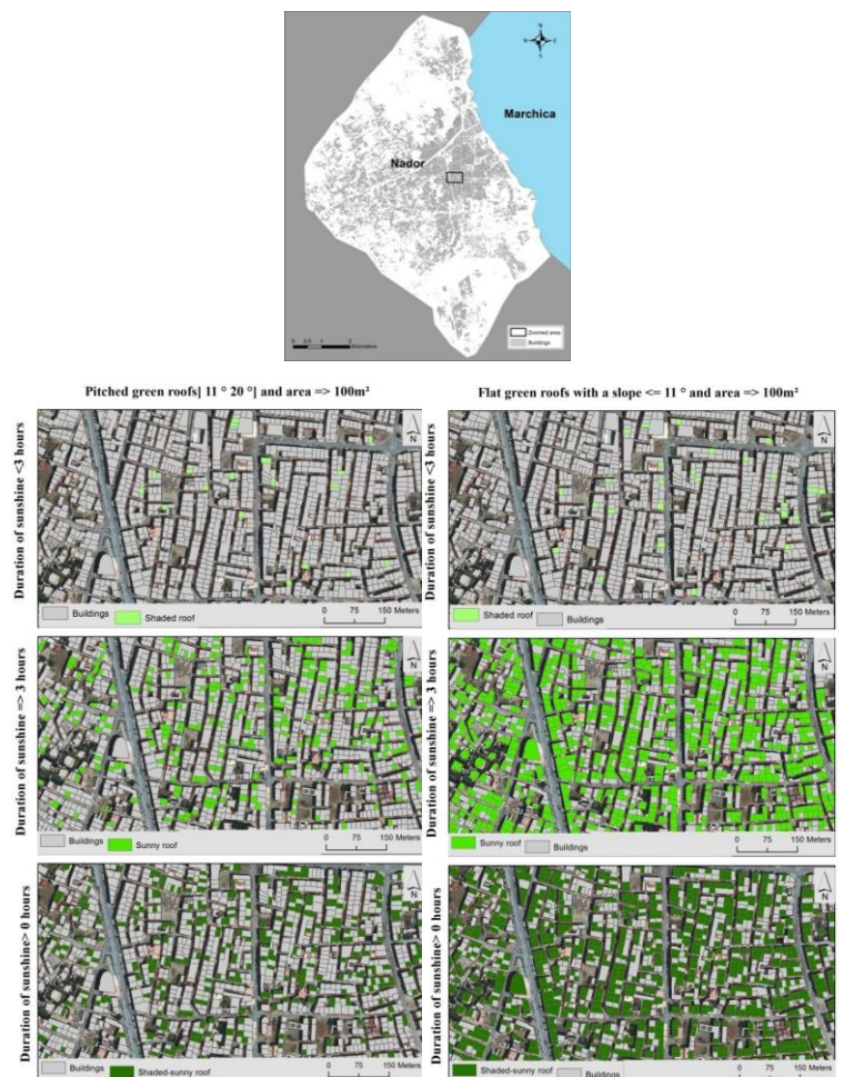
Figure 4. Potential green zone on the roof depending on the inclination of the roof and sunshine criteria
