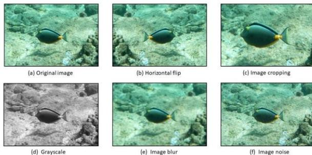
**Figure 3.** Some examples of the data augmentation step: (a) original image, (b) horizontal flip, (c) image cropping, (d) grayscale, (e) image blur up to 10px, (f) image noise up to 10% of pixels
