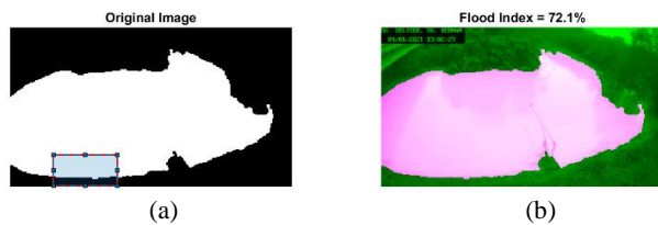
Figure 4. The flood index for the image of 4th of August 2021. (a) The ROI contains more white pixels than black. (b) The flood index computed was 72.1%.
