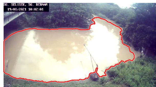
Figure 3. The segmentation result that extracts water from the background.
