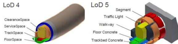
**Figure 4.** LoDs of tunnel extracted from Borrmann et al., 2013, p.80.
