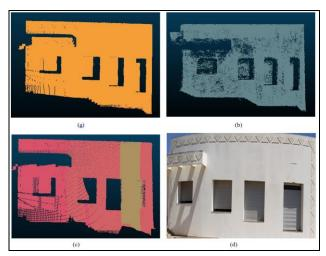
**Figure 5**. Extraction of windows from different point clouds: (a) from TLS, (b) from Drone, (c) from merged point cloud, (d) origin image
