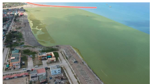
Figure 4. Aerial photo of the study area. Yellow area highlights the accumulation of sand sediments.
