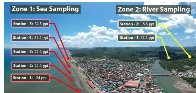
Figure 7. Measured salinity concentration of different locations on the river and nearshore, where the reclamation shall be done.
