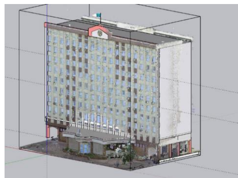
Figure 10. Point cloud in SketchUp software loaded using the Undet module.
