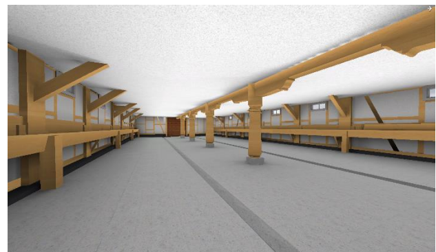
Figure 8. BIM model of the ground level of the building with custom wooden structures.
