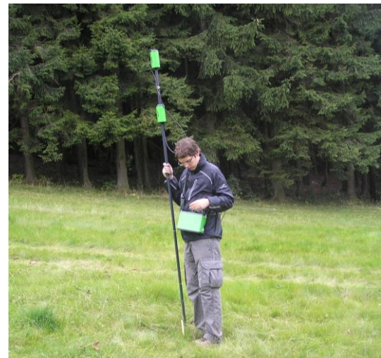
Figure 3. The gradient magnetometer in the field.
