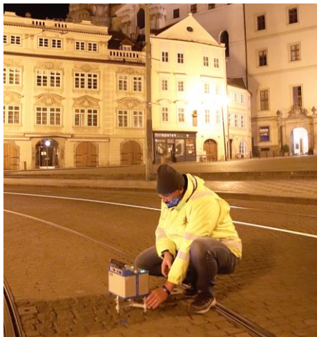
Figure 1. The gravity measurement in the centre of Prague
