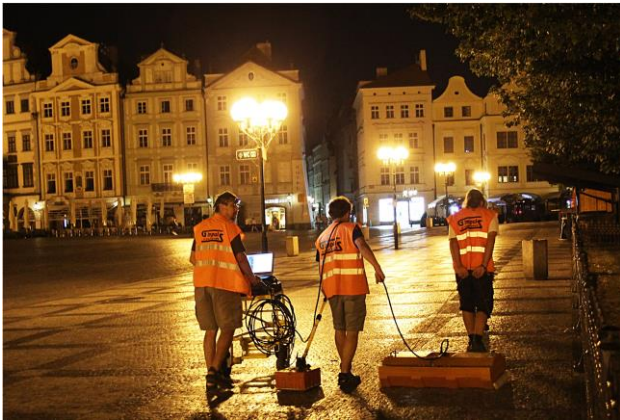
Figure 14. The GPR equipment with two antennas (see boxes on the pavement) in the work.
