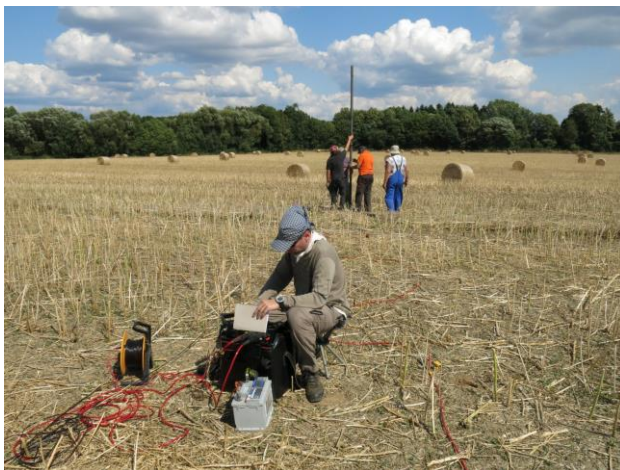
Figure 18. The seismic measurement in a field. In the front is seismic equipment, in background is seismic resource (impact mechanism).
