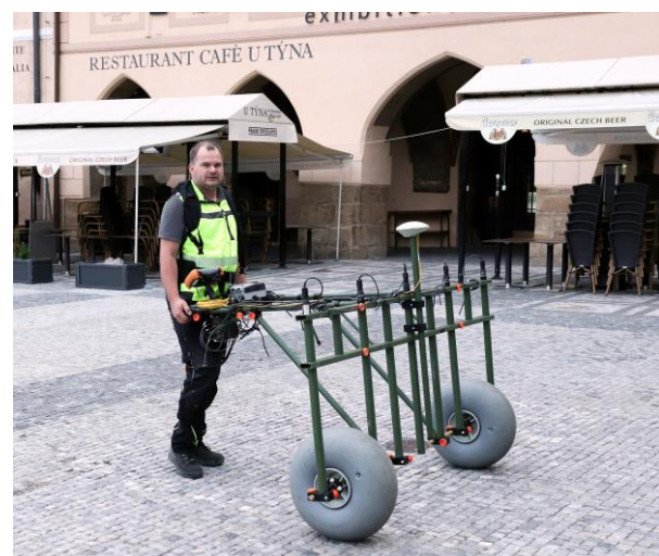
Figure 4. The multichannel magnetometer for archaeological or pyrotechnical prospection
