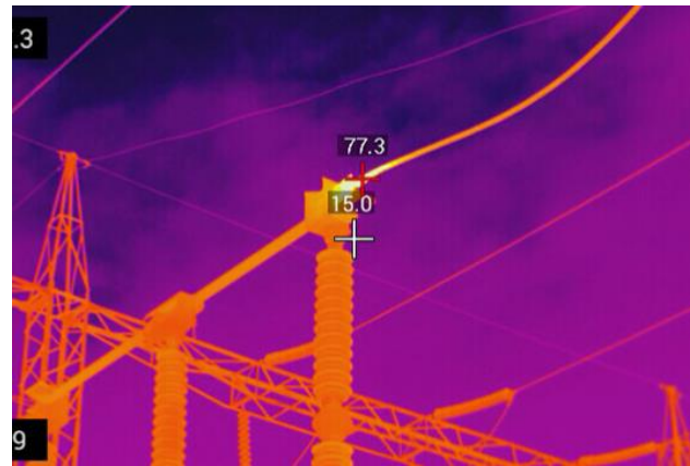
Figure 19. The snap of distribution net by thermo camera. The temperature 77.3 and 15 is reading in ^{\circ}\text{C} .
