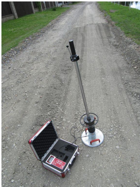
Figure 23. The equipment for the impact load test with a light dynamic plate. By ArtepGeo.
