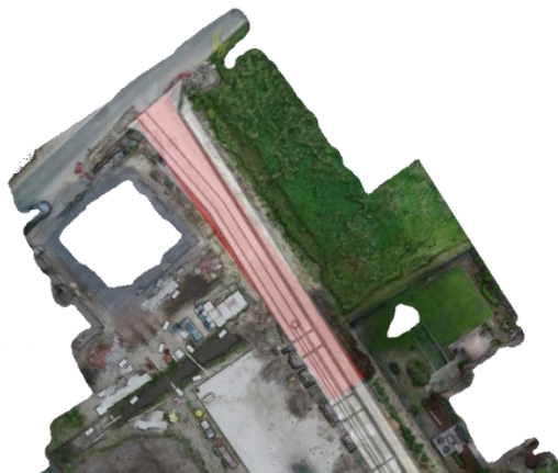
Figure 8. Detection of sub-foundation out of a mesh compared to the as -design BIM. The sub-foundation is not finished.
