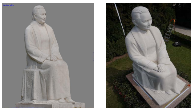
Figure 4. 3D modelling in process and the final digital model, with its perspective distortion eliminated, comparing with the real photo of the statue. (Source: Zhong Tang)
