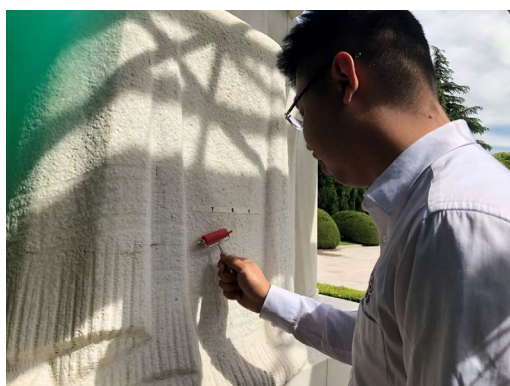
Figure 12. Conducting the chalking evaluation test on the side of the statue in May 2019. (Source: Tongji-ACL)
