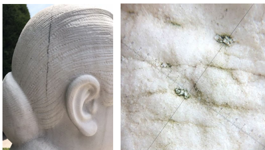
Figure 2. Deteriorations on the statue: cracks, chalking, moss, old paint photo taken in May 2018. (Source: Tongji-ACL)
