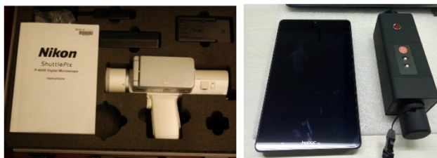
Figure 8. The Nikon hand-held microscope and the crack width observation instrument. (Source: Tongji-ACL)
