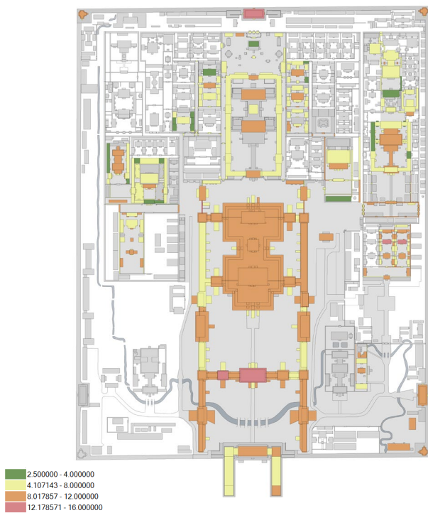
Figure 7. The overall deterioration condition of masonry.
