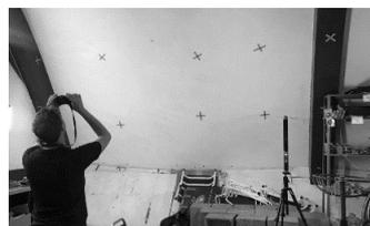
Figure 6. One of the Canadian students collecting interior photogrammetry data of the pavilion using a handheld DSLR camera.
