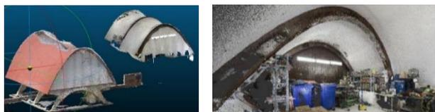
Figure 11. **Left:** Two separate interior and exterior Point cloud data of the pavilion in CloudCompare software. **Right:** Shows interior point cloud data in Agisoft Photosca Software. . (Produced by Rajabzadeh, 2019)
