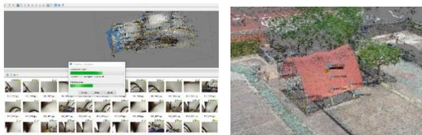
Figure 13. **Left:** Photo aligning process in Agisoft Photoscan Software using the target points. **Right:** Dense cloud of the whole site created in Agisoft Photoscan Software (Produced by Rajabzadeh, 2019)
