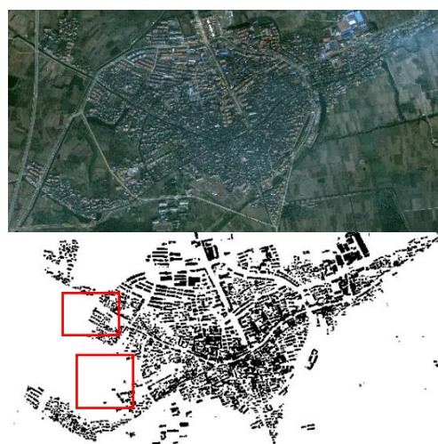
(a) Remote sensing image and semantic segmentation image of Fenghui Town in 2007
