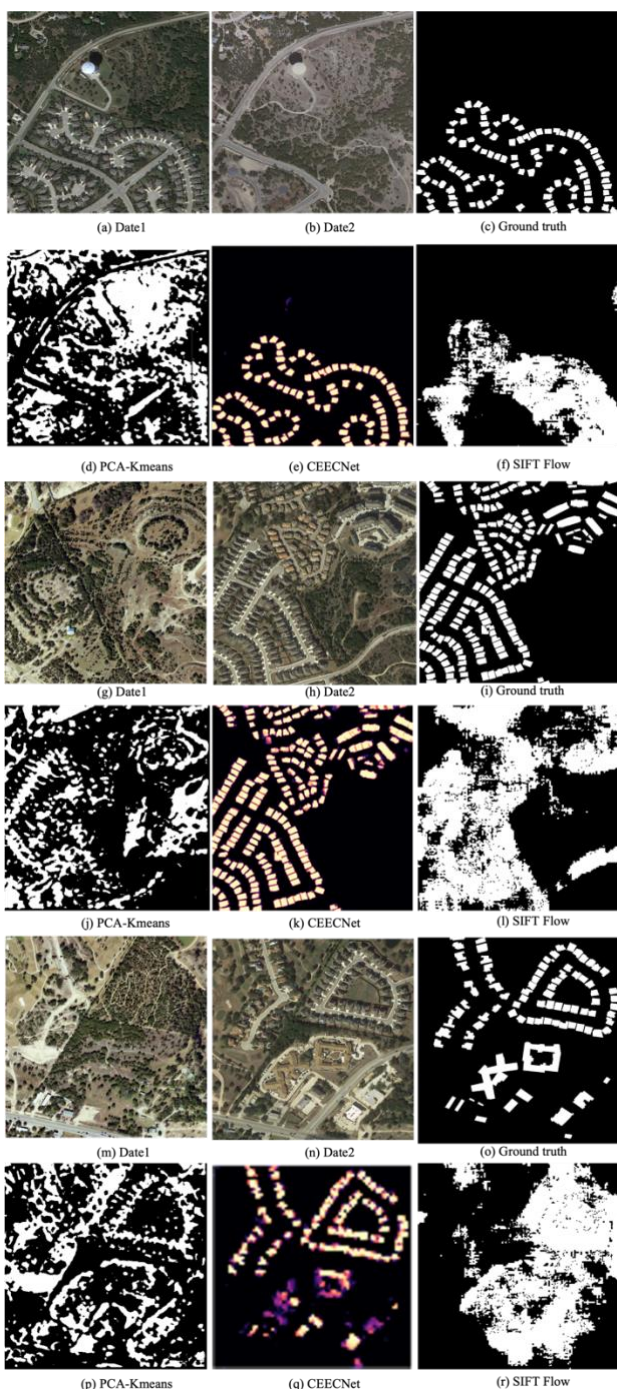
Figure 7. Results each odd row is the pair of input images and their ground truth. Each even row is the results of PCA-Kmeans, CEECNet and SIFT flow respectively.
