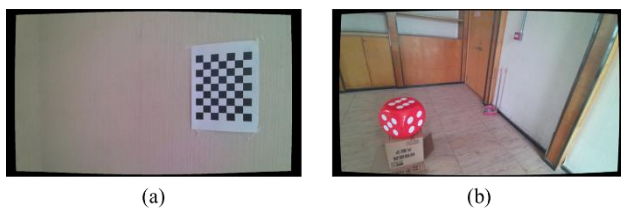
Figure 7. Undistorted images after radial distortion removal. (a) Zhang's checkerboard method; (b) our method.
